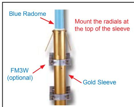
1. Attach the four radials to the top of the sleeve using the four bolts and lock washers "radials tilted downwards".
